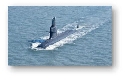
• **Propulsion:** Diesel-electric propulsion; Air-independent propulsion (AIP)
