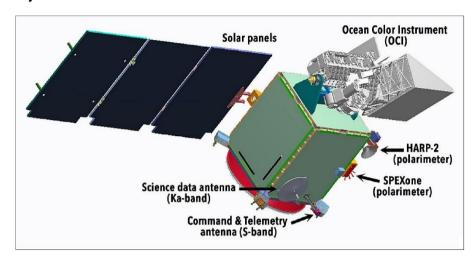
PACE mission will also feature two advanced polarimeters, the Spectropolarimeter for Planetary Exploration (SPEXone) and the Hyper Angular Research Polarimeter (HARP2).
