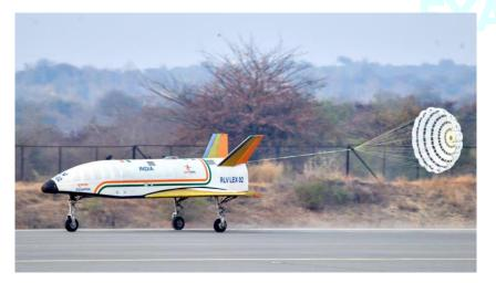
• With the RLV-LEX-02, ISRO has re-validated its indigenously developed technologies in areas such as navigation, control systems, landing gear, and deceleration systems, which are essential for performing a high-speed autonomous landing of a space-returning vehicle".
