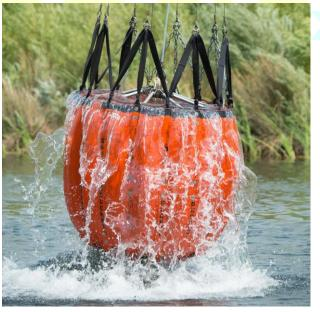
• One of its key features is that it can be quickly and easily filled. The bucket can be **filled from various sources**, including lakes and swimming pools, which allows firefighters to swiftly refill it and return to the target area. Bambi Bucket
