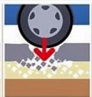
Weight of traffic collapses the road surface into the hole
