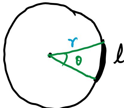
$$\theta \text{ (in radian)} = \frac{\text{length of arc}}{\text{radius}} = \left( \frac{l}{r} \right)$$
