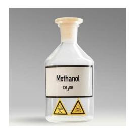
• **Now, methanol has a boiling point** of 64.7 °C, lower than that of ethanol 78.37 °C. During distillation, when the mixture reaches 64.7 °C, the pot collecting concentrated alcohol begins to fill up with a highly toxic chemical. This must be discarded for the end product to be safe.
