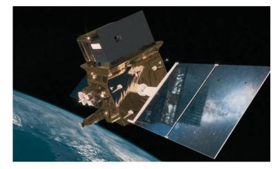
• The satellite will have two main payloads: a Thermal Infra-Red (TIR) sensor from CNES and a Visible, Near Infra-Red, and Short Wave Infra-Red (VNIR-SWIR) sensor made by ISRO. These high-tech tools will make it easier to map the surface temperature with great detail and analyze the surface reflectance in great detail. Both of these are key to collecting important biological and atmospheric data.
