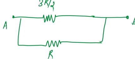
for 2 resistors in parallel, equivalent resistance =
