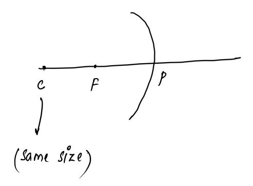
An enlarged image is formed when object is between c and P.
