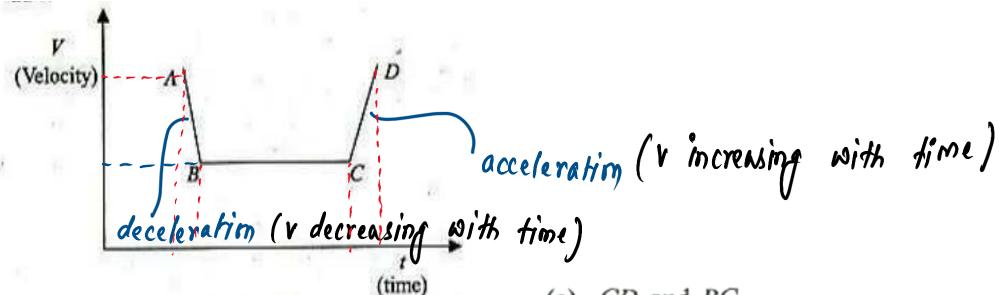
In the given velocity (V) versus time (t) graph, accelerated and decelerated motions are respectively represented by line segments
