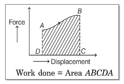
Work done in displacing any body under the action of a number of forces is equal to the work done by the resultant force. In equilibrium (static or dynamic), the resultant force is zero, therefore resultant work done is zero.
