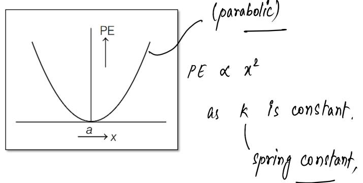
If a spring of spring constant k is stretched through a distance x,
