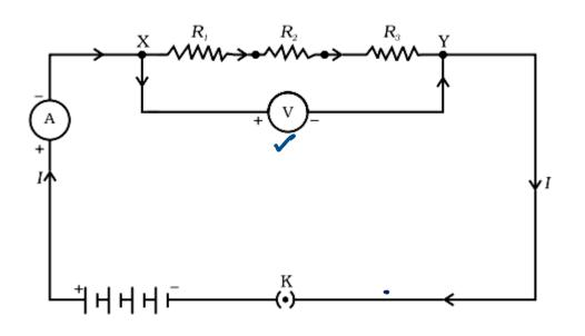
$$R = R_1 + R_2 + R_3$$
