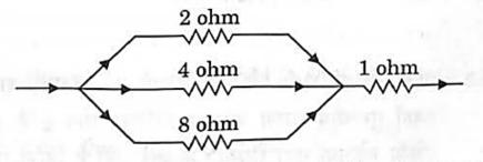
The total electrical resistance in the given part of the electric circuit is
