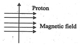
A proton enters a magnetic field at right angles to it, as shown above. The direction of force acting on the proton will be
