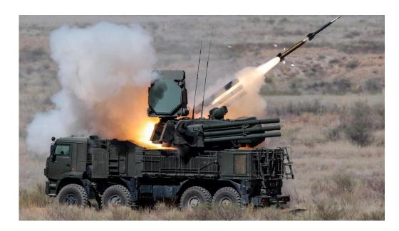
The Pantsir-S1's capabilities include engaging targets within a range of 1,200 to 20,000 meters using missiles, and 200 to 4,000 meters with gun weapons. The altitude range for missiles is from 15 to 15,000 meters, while guns can engage targets between 0 to 3,000 meters.
