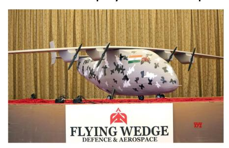
The UAV can operate at a maximum speed of **370 kmph** (200 knots), with an endurance of **12-20 hours** and a ground control station range of **200 km**.
