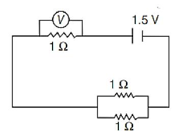
What should be the reading of the voltmeter V in the circuit given above? (All the resistances are equal to  $1 \Omega$  and the battery is of 1.5 V)
