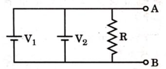
where value of  $V_2$  = 5 V. The internal resistances of both the batteries are 0·1  $\Omega$ . The current through the resistance R is about:
