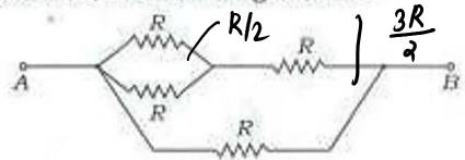
Which one of the following is the value of the resistance between points A and B in the circuit given above?
